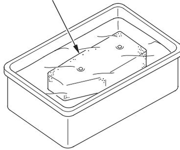
5. Dip the air cleaner element in clean engine oil, then squeeze out all excess oil. The engine will smoke when started if too much oil is left in the filter.
