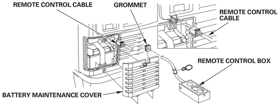
7. To avoid accidentally unplugging the remote control cable, secure the cable to the generator frame with a cable tie as shown.
