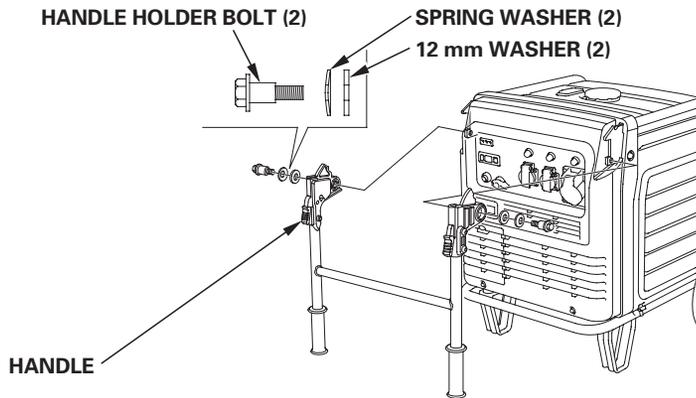
Operation must be checked after attaching a handle.
