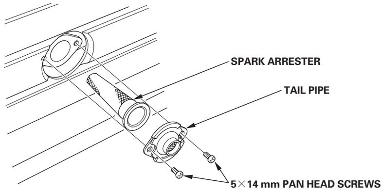
2. Use a brush to remove carbon deposits from the spark arrester screen.
