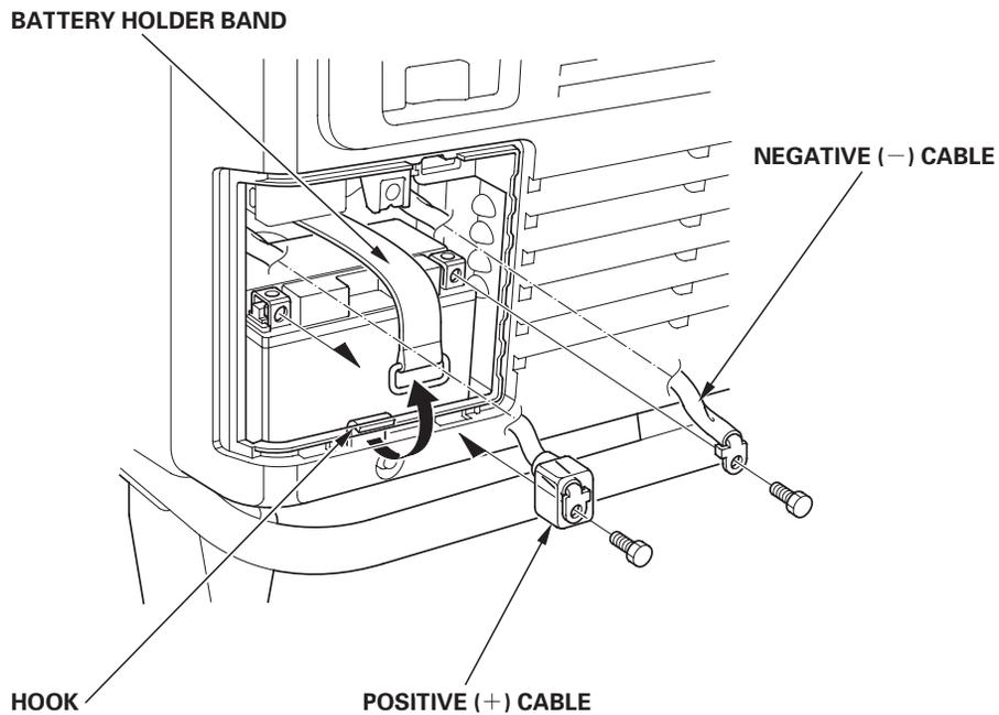
6. Remove the battery from the battery tray.
