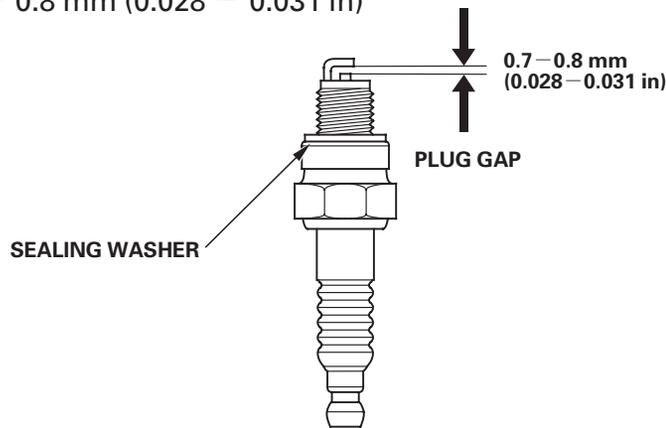
7. Install the spark plug carefully, by hand, to avoid cross-threading.
